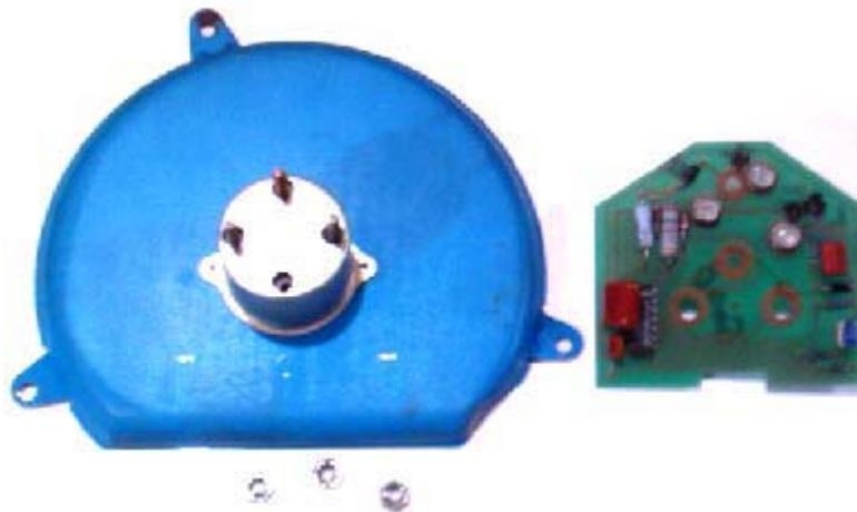
The new board may look a little differently than the one you are replacing. This should not be cause for concern. Older reproduction boards used a red washer between the tach board and the metal can. Currently, only imported boards use these washers. Our boards do not use or need insulating washers for installation. Only boards made in the USA are made correctly and do not require insulating washers.
