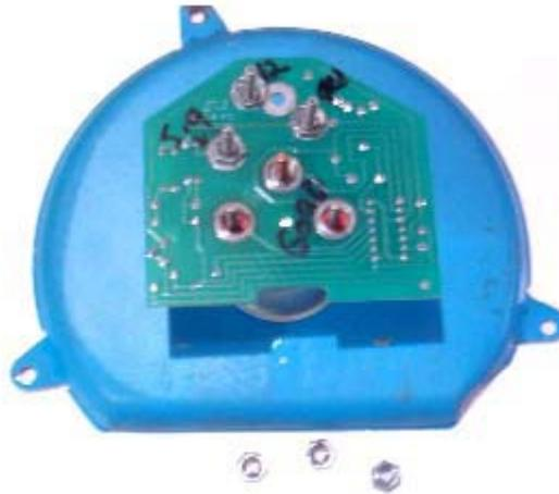
Attach the three board nuts as shown below and you are now finished.
